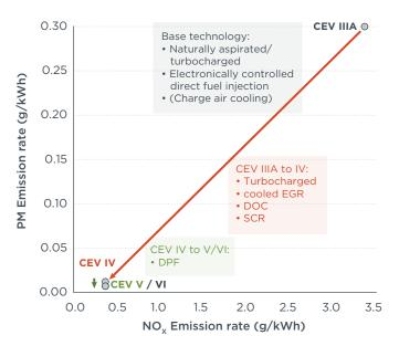
Figure 14. Projected technology pathway for diesel engines used in construction equipment between 75 and 130 kW (100 and 175 hp).
