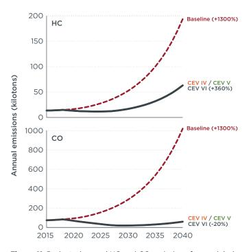
**Figure 11**. Projected annual HC and CO emissions for modeled construction equipment emission-control scenarios. Values on the right side of the plots show the percentage change in emissions between 2015 and 2040 for each scenario.
