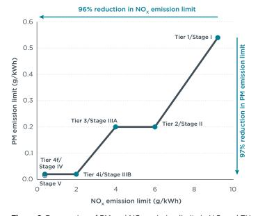
**Figure 2**. Progression of PM and  $NO_x$  emission limits in U.S. and EU non-road engine emission-control programs (130 kW engine).
