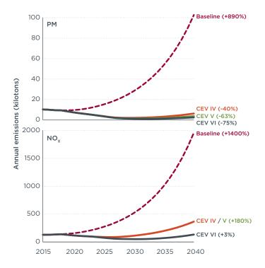
**Figure 10**. Projected annual PM and  $NO_x$  emissions for modeled construction equipment emission-control scenarios. Values on the right side of the plots show the percentage change in emissions between 2015 and 2040 for each scenario.
