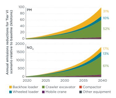
Figure 12. Annual PM and NO, emission reductions for construction equipment in the CEV VI scenario relative to baseline, disaggregated by equipment type. Percentages show relative share of cumulative emission reductions between 2020 and 2040 for select equipment types.
