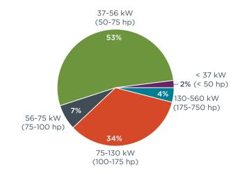
Figure 9. Estimated engine power distribution for construction equipment in India, 2014.13
