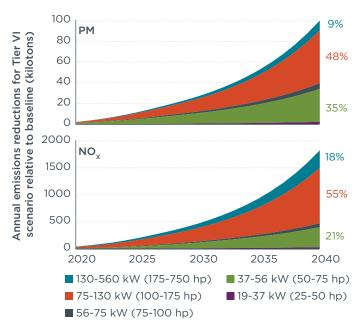
Figure 13. Annual PM and NOx emission reductions for construction equipment in the CEV VI scenario relative to baseline, disaggregated by engine power class. Percentages show relative share of cumulative emission reductions between 2020 and 2040 for select power classes.
