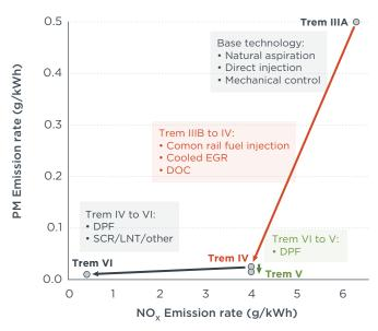
Figure 8. Projected technology pathway for agricultural tractor engines between 19 and 37 kW (25 and 50 hp).
